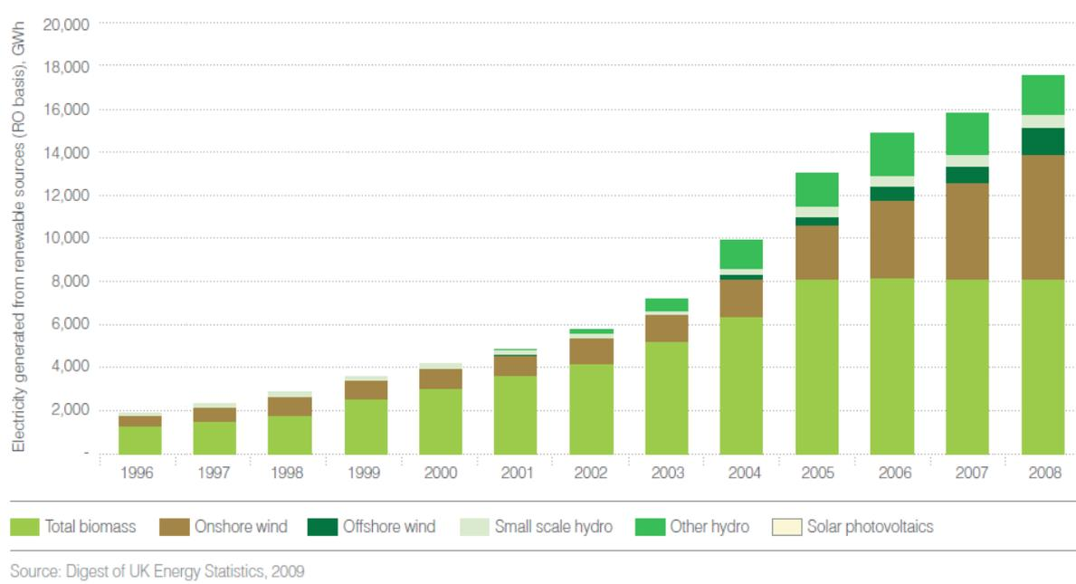
Biomass has higher availability than most renewables. This is known as the load factor of a generating technology. A dedicated biomass plant, for example, has a load factor of up to 90%, with 10% downtime for maintenance. The intermittent nature of other renewable technologies leaves them trailing.
